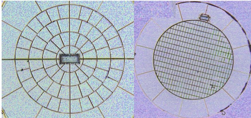
Figure 2: Picture of a 143 GHz (*left*) and of a 217 GHz spiderweb bolometer (*right*), with a temperature sensor in the centre and at the upper edge respectively.
