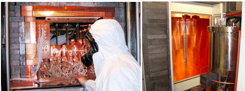
Figure 6: Examples of detector shielding, DAMA detector (left) and XENON100 detector (right).
