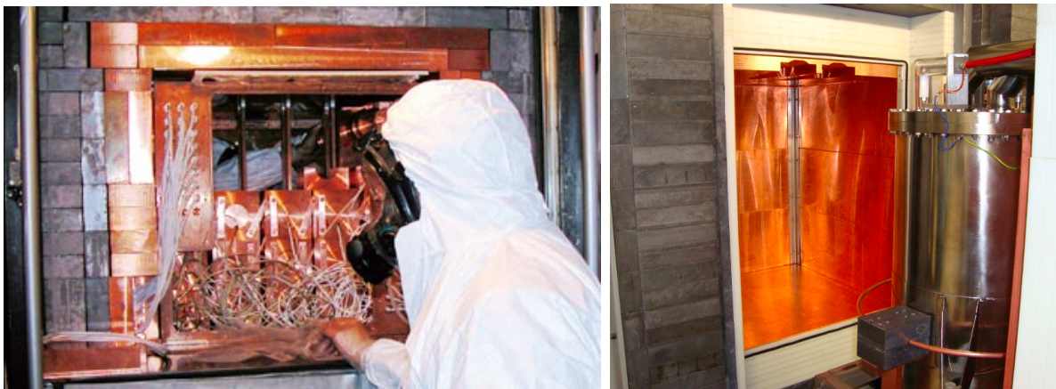
Figure 25. Examples of detector shielding using layers of lead, copper and polyethylene: DAMA detector (left) and XENON100 detector (right).
