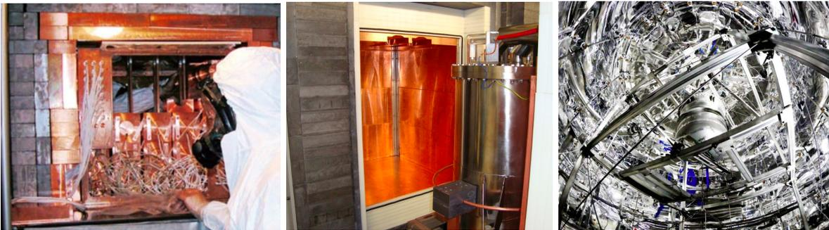
**Figure 7.** Examples of detector shielding: DAMA detector (left), XENON100 detector (middle) and XENON1T water tank (right). Figures from the corresponding collaborations.
