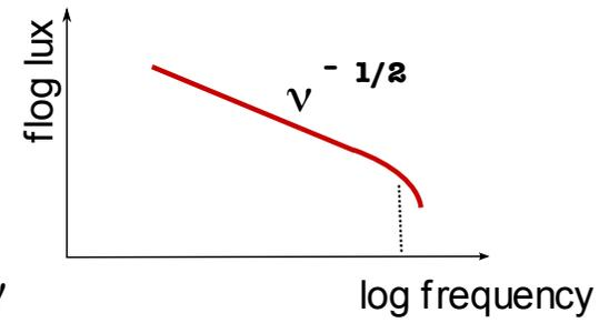
Resultant synchrotron spectrum
