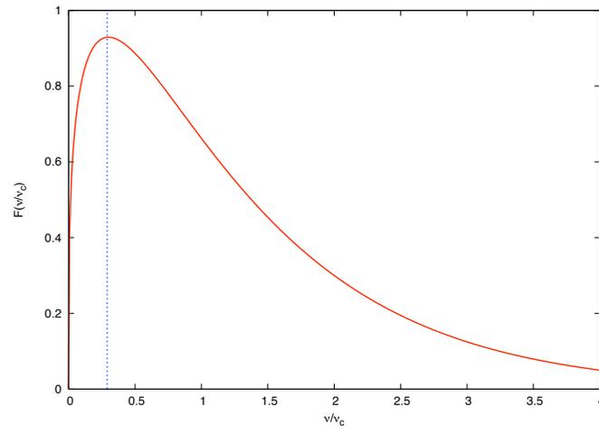
Figure 1:  $F(\nu/\nu_c)$  as function of frequency  $\nu/\nu_c$ . The spectrum has a maximum at  $\nu_{max} = 0.29\nu_c$ .
