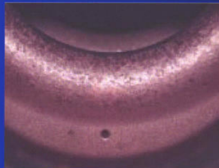
Iris damage at high gradients
