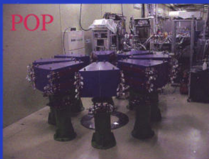
Proof of Principle (POP) FFAG tested at KEK in June 2000
