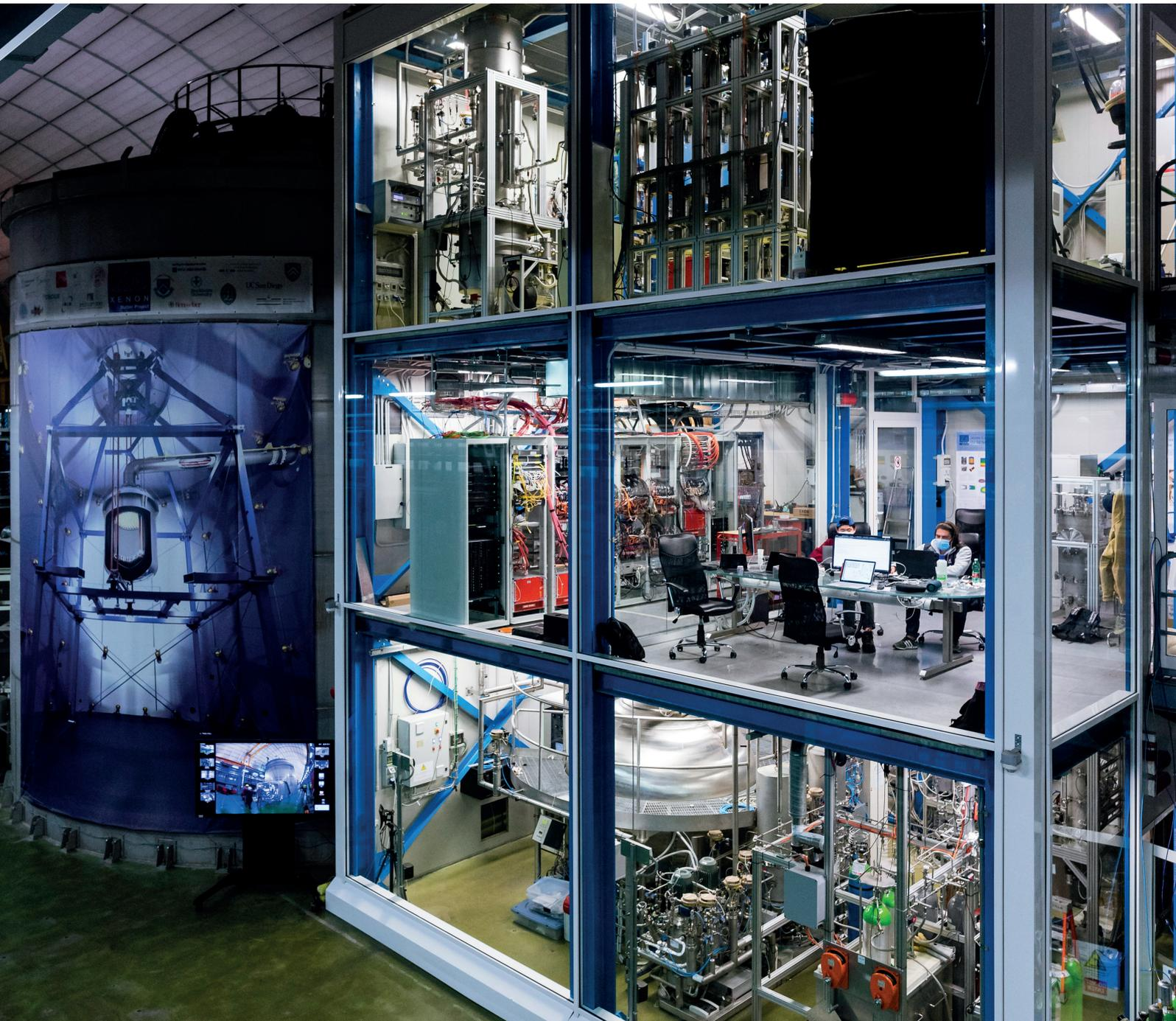
*Cover: The XENONnT experiment underground in the Laboratori Nazionali del Gran Sasso (LNGS) in Italy with the three-storey service building and the water tank containing the detector and veto systems.*
