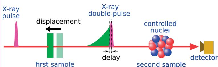
Schematic setup for the coherent control of nuclear dynamics.
