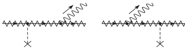
Feynman graphs for laser-assisted Bremsstrahlung. The zig-zag line represents an electron embedded in the laser field, the broken line the interaction with the nucleus and the wavy line the emitted X-ray quantum.
