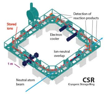
Overview of the Cryogenic Storage Ring (CSR) with experimental sections for neutral atom injection and electron cooling.
