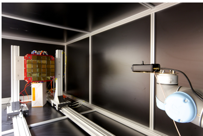
Automated performance test of the CHEC prototype in the laboratory with the aid of a laser, mounted on a robot.
