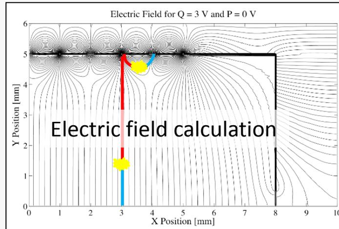
ZIP with interleaved electrodes: iZIP
