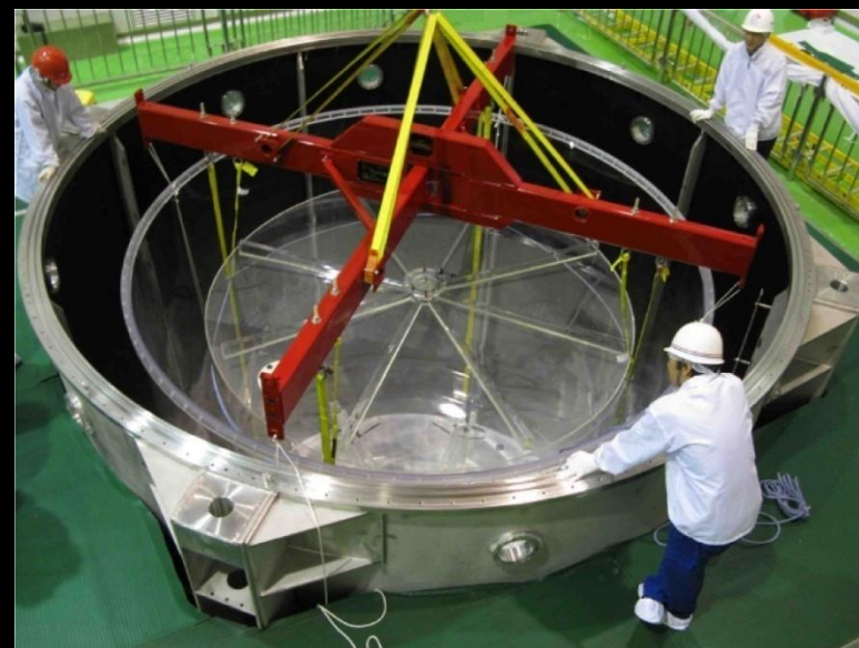
Detector mechanics: 5-m SST vessel, 4-m and 3-m acrylic vessels in surface assembly hall
