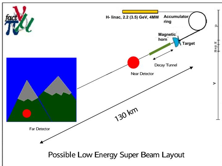
The SPL SuperBeam experiment is conceptually identical to T2HK: generate a conventional neutrino beam and fire it to a megaton water Cerenkov detector. So why don't simply take the default description of T2HK in Globes and adapt it to the different beam?:
