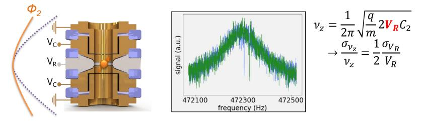
$\Delta v_{z,I}({}^{1}H^{+}) \approx 100 \text{mHz} \rightarrow 80 \text{nV/V}_{0}$  to detect a spin flip with a fidelity of 80%  $\Delta v_{z,I}({}^{3}He^{2+}) \approx 25 \text{mHz} \rightarrow 20 \text{nV/V}_{0}$
