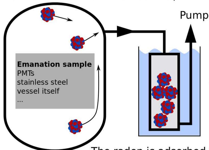
The radon is adsorbed while the carrier gas is pumped out.
