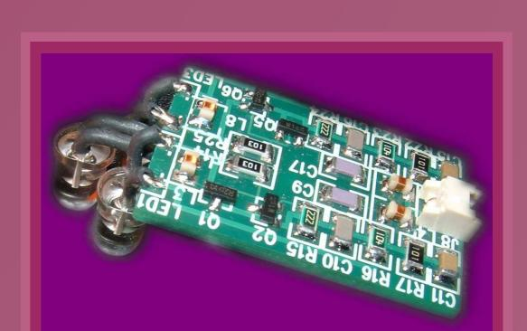
The LED pulser, designed at Sheffield University, is the 'heart' of our flat-fielding system. For our specific purposes, we have integrated three pulsers into the flat-fielding circuit (see picture).
