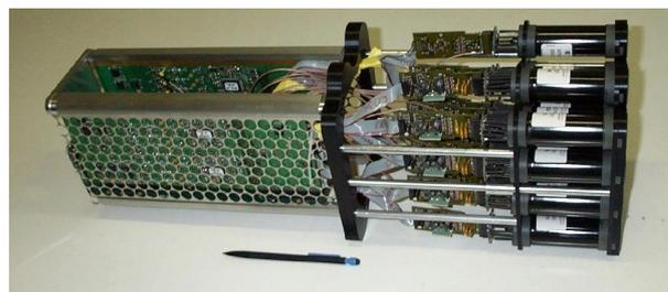
**Fig. 4.** A “drawer” contains 16 PMTs, their individual HV supplies, as well as the analog and digital electronics and the trigger circuitry.
