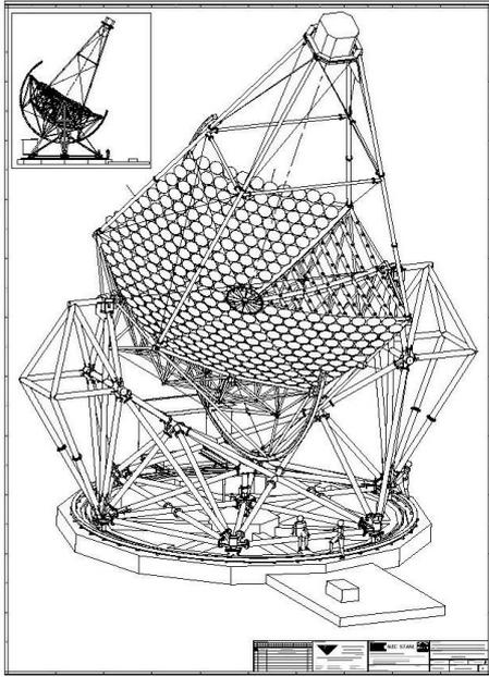
**Fig. 1.** One of the H.E.S.S. telescopes; on one section of the dish, mirrors are removed to show the support structure.
