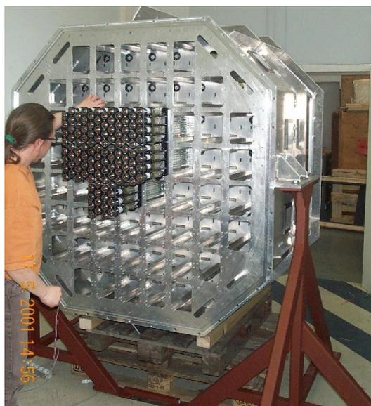
**Fig. 3.** Camera body, with some the “drawers” inserted.
