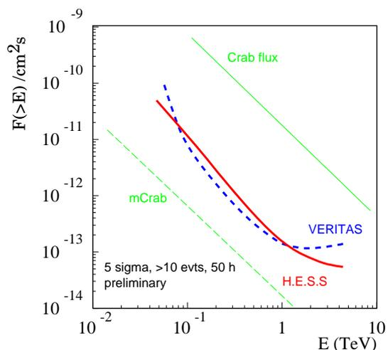
**Fig. 5.** Minimal detectable flux as a function of energy threshold, for 50 h of observation time. Also shown is the sensitivity quoted in the VERITAS proposal, and for comparison the Crab flux levels.
