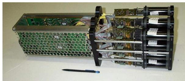
**Fig. 4.** A “drawer” contains 16 PMTs, their individual HV supplies, as well as the analog and digital electronics and the trigger circuitry.
