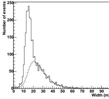
**FIGURE 2.** 3D-width distributions from Crab data. (a) Solid-line histogram: events for a region close to the source ( $\theta < 0.05 \text{ deg}^2$ ). (b) Dotted-line histogram: events in a region that excludes the source ( $\theta^2 > 0.2 \text{ deg}^2$ ). Both histograms are normalized to the same number of events with widths greater than 40 m.
