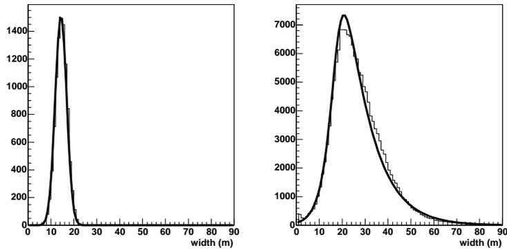
**FIGURE 5.** “A posteriori” 3D-width distributions for gamma-rays (left) and hadrons (right), compared to functions  $g(x)$  and  $b(x)$  used in the method.
