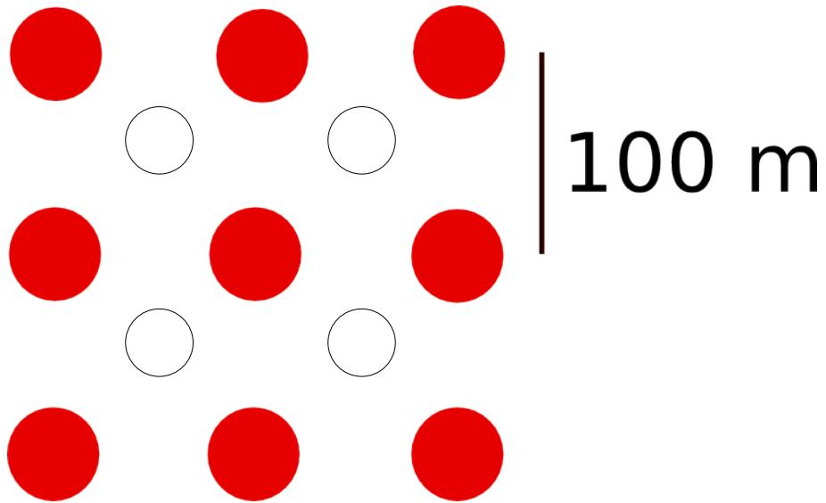
9 telescopes of 23 m diameter,  $f=28$  m, 80% mirror reflectivity, 2029 pixels of  $0.1^\circ$ , HESS-I Q.E.
