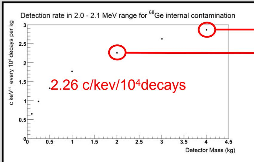
**26% more events registered in the RoI in a 4 kg detector than in a 2 kg one for  $^{68}\text{Ge}$  internal contamination.**
