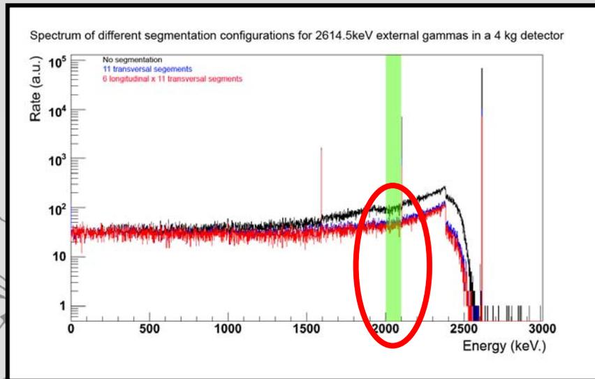
Up to **98 out of 100** background events coming from  $^{60}\text{Co}$  internal contamination can be rejected applying segmentation and anticoincidence techniques.
