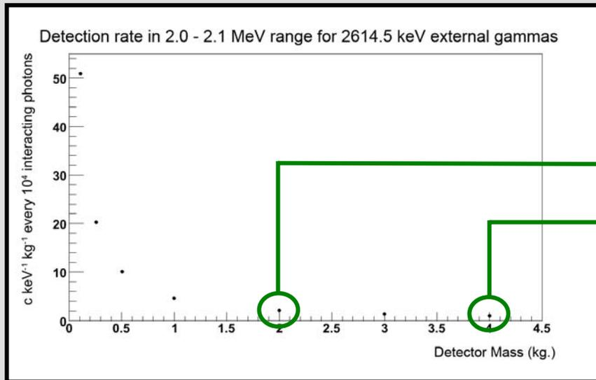
**54% less events registered in the RoI in a 4 kg detector than in a 2 kg one for 2614.5 keV external photons.**
