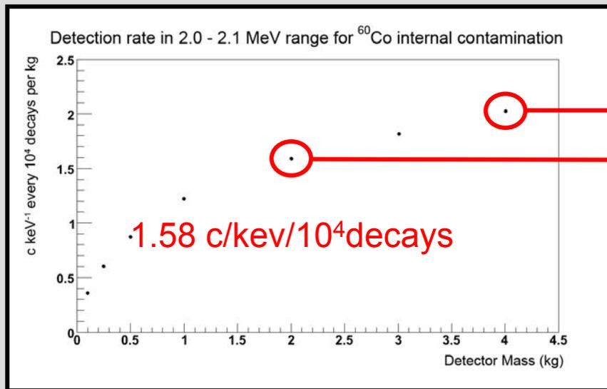
**28% more events registered in the RoI in a 4 kg detector than in a 2 kg one for  $^{60}\text{Co}$  internal contamination.**
