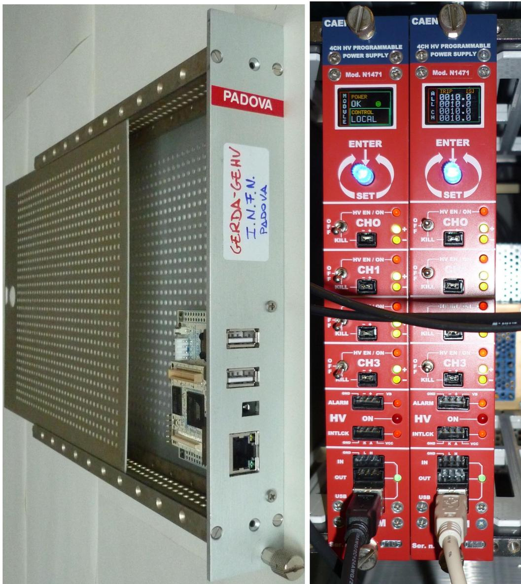
Figure 10: The NIM module containing a small board (left side) controlling the HV CAEN N1471 modules (right side) via USB/serial interface.
