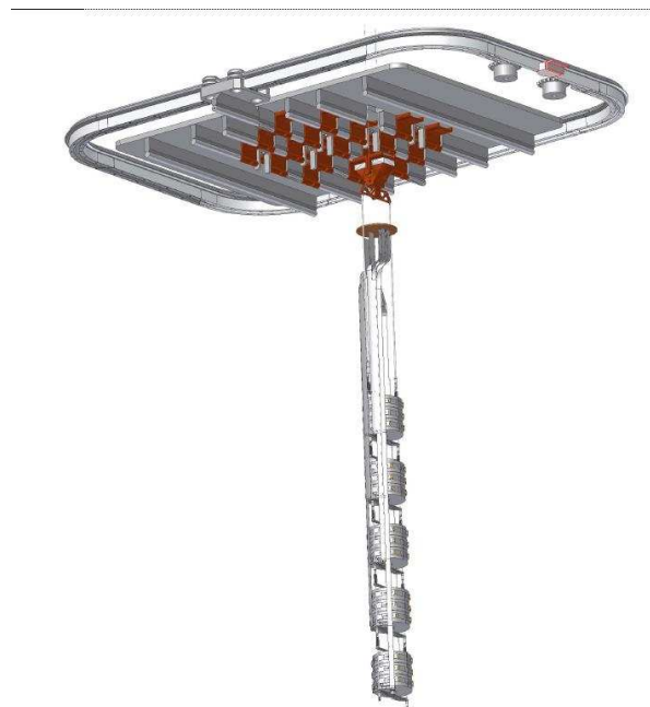
Figure 23: The rail system to position and lower individual strings.
