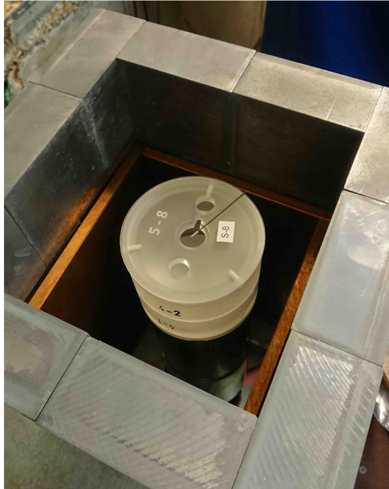
FIGURE 4.2: Measurement set-up at the HADES facility in Mol, Belgium. It consists of a lead castle surrounding a cryostat consisting of an aluminum cap and a copper holder which carries an IC detector cooled by a coldfinger from below. Here, the ^{228}\text{Th} source is in a radially centered position 10 cm above the cryostat.
