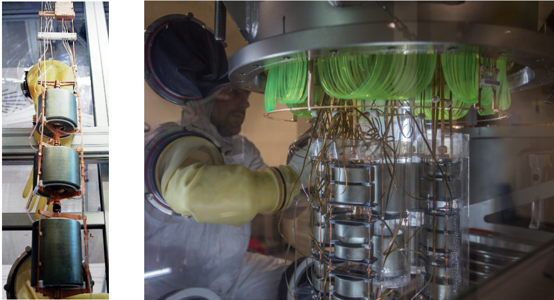
FIGURE 3.2: Left: Central string of the GERDA array, featuring the 3 natural non-enriched coaxial type detectors GTF112, GTF32, and GTF45. Right: Position of the central string surrounded by the other 6 strings in the clean room before lowering into the cryostat.
