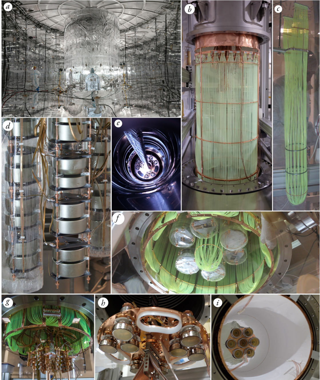
Figure 2.6: Various pictures of the GERDA Phase II setup, taken during the upgrade works. a) the muon veto instrumentation inside the water tank; b) the light guiding outer fiber shroud; c) the central fiber shroud; d) Phase II array closeup, BEGe detector strings with their holder mounting and WLS mini-shroud are visible; e) the array being lowered into LAr; f) the end cap of the central fiber shroud is visible from below the assembled array; g) the electronics front-end; h) the top PMTs and holes for calibration sources; i) the bottom PMTs inside the Tetratex ® -coated copper shroud.
