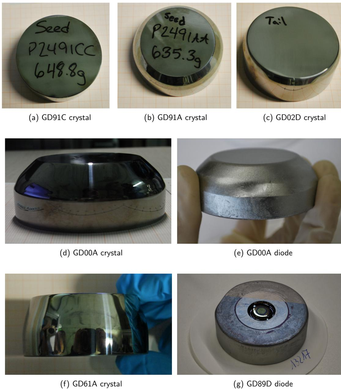
Figure B.1 Examples of a regular (GD91C) and irregular shaped BEGe detectors before and after diode conversion.
