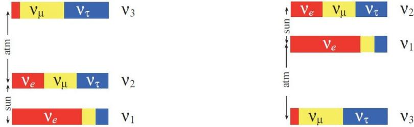
Figure 2.1 Two different scenarios of neutrino mass patterns deduced from oscillation experiments. Left: normal mass hierarchy ( $\nu_1 < \nu_2 < \nu_3$ ); right: inverted mass hierarchy ( $\nu_3 < \nu_1 < \nu_2$ ). The flavor composition of neutrino mass eigenstates is illustrated with red for the  $e$  part, with yellow for the  $\mu$  part and with blue for the  $\tau$  part. From [12].
