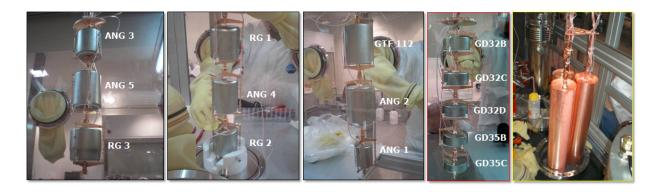
Figure 3.2: GERDA Phase I detectors mounted in the strings. Figure from left to right represents different detectors mounted in different strings. The closed-end coaxial HPGe detectors were mounted in the first three strings; all the BEGe detectors were mounted in a single string. The right most figure shows that each string was enclosed by a radiopure copper mini-shroud to mitigate  ${}^{42}$ K background (see Section 3.3).
