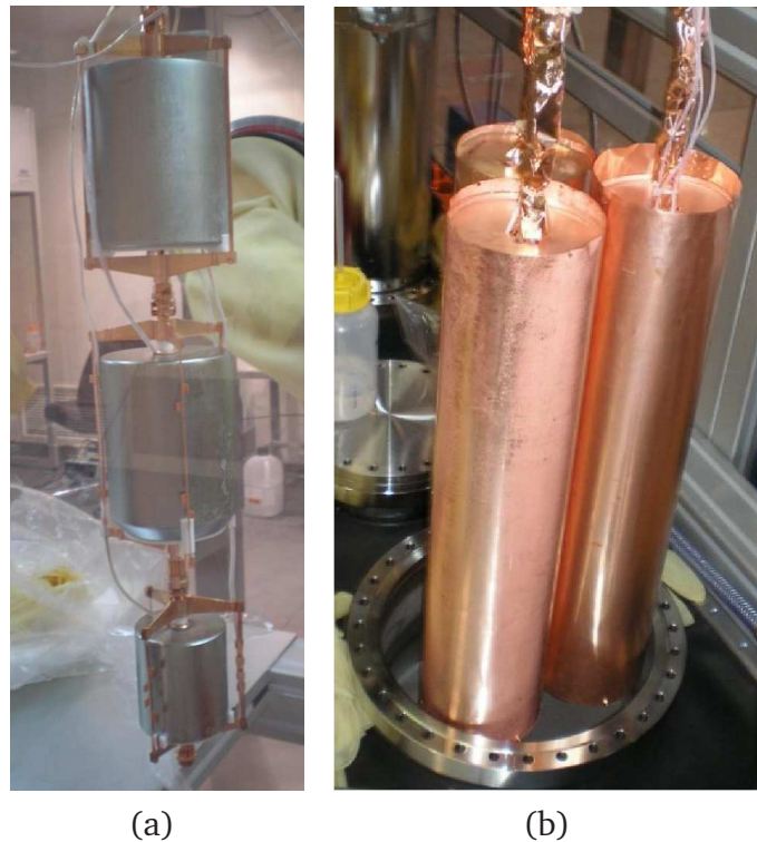
Figure 6.1: (a) String of three Phase I detectors in their low mass holders. (b) Three detector strings contained in their minishrouds.
