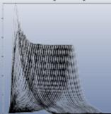
simulated pulse shapes after convolution with impulse response
