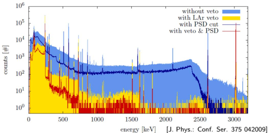
Pulse shape analysis combined with LAr-scintillation (in LArGe setup): measured suppression factor of  $(5.2 \pm 1.3) \cdot 10^3$  at  $Q_{\beta\beta}$  for close Th-228
