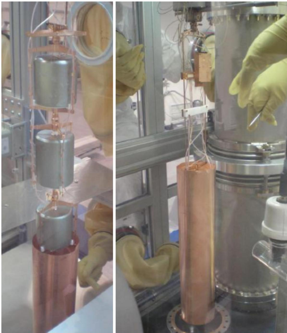
Figure 4.4: Left: a string of three enrGe detectors is inserted into the mini-shroud. This work is performed in the glove box of the clean room. Right: closed detector string and 3-channel preamplifier inside a copper box about 30 cm above the string. The connections between the preamplifier and detectors are made with Teflon insulated copper strips that are tightly fixed to prevent microphonics. In the background, part of the 3-string lock is visible.
