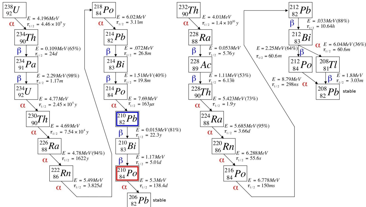
$^{210}\text{Pb}$  surface contamination  $\Rightarrow$  expect 5.3 MeV alphas from  $^{210}\text{Po}$  at a constant rate
