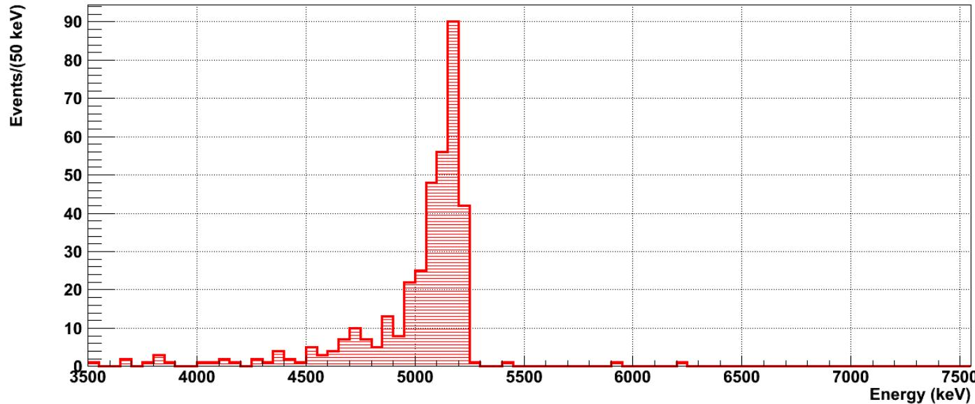
**Assumption:** Majority of high-energy events come from  $^{210}\text{Po}$   $\alpha$ -decays ( $E = 5.3$  MeV) at the surface, due to an initial  $^{210}\text{Pb}$  surface contamination.
