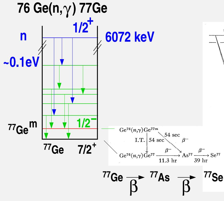
FIG. 6. Decay scheme of  $^{77}\text{Ge}$ .
