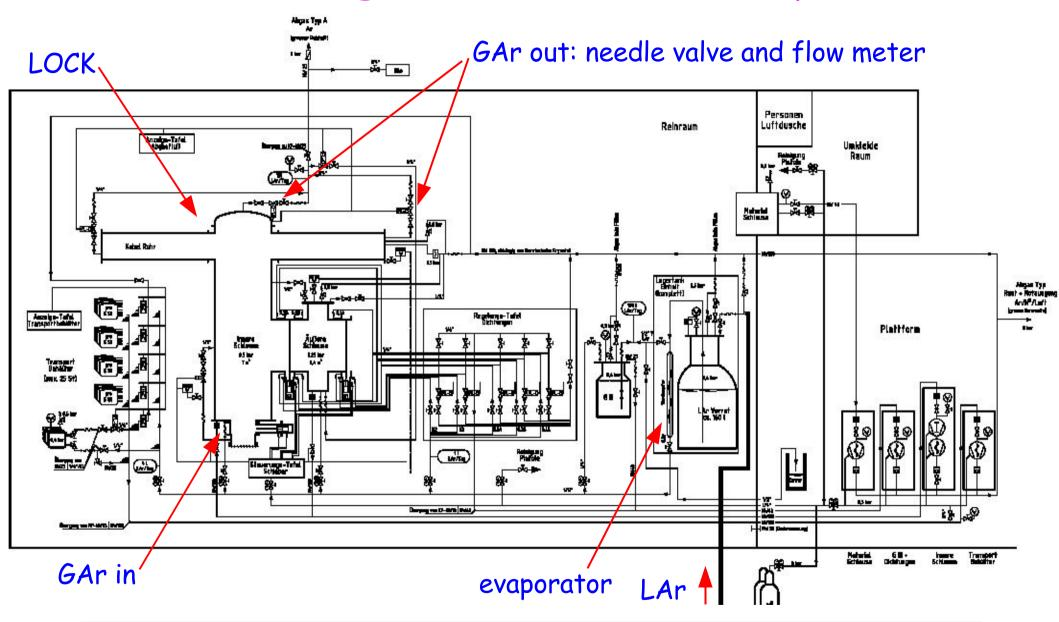
(variable) flow of GAr for Rn purging will modify gas pressure of cryostat
