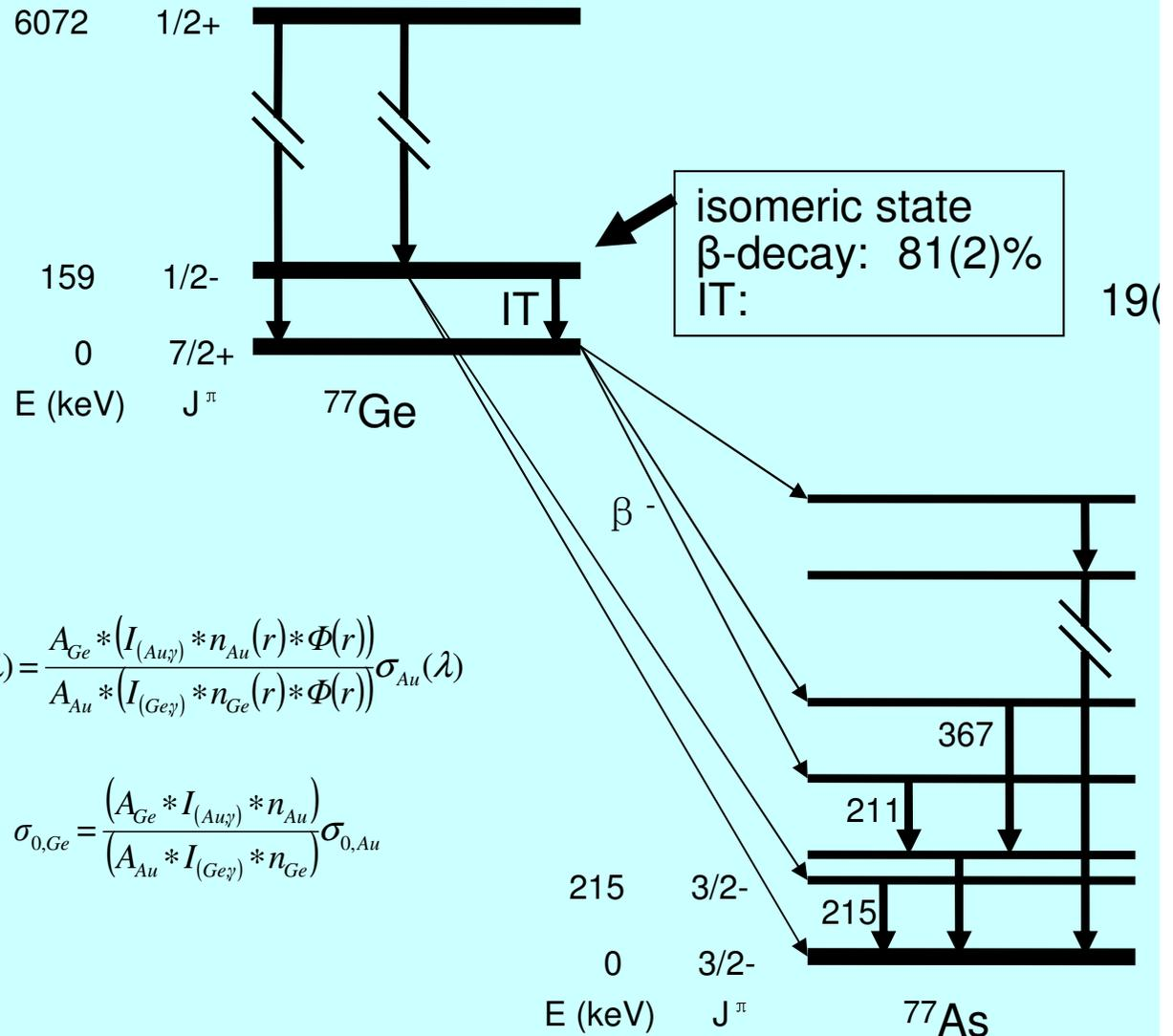
$$\sigma_{Ge}(\lambda) = \frac{A_{Ge} * (I_{(Au\gamma)} * n_{Au}(r) * \Phi(r))}{A_{Au} * (I_{(Ge\gamma)} * n_{Ge}(r) * \Phi(r))} \sigma_{Au}(\lambda)$$
