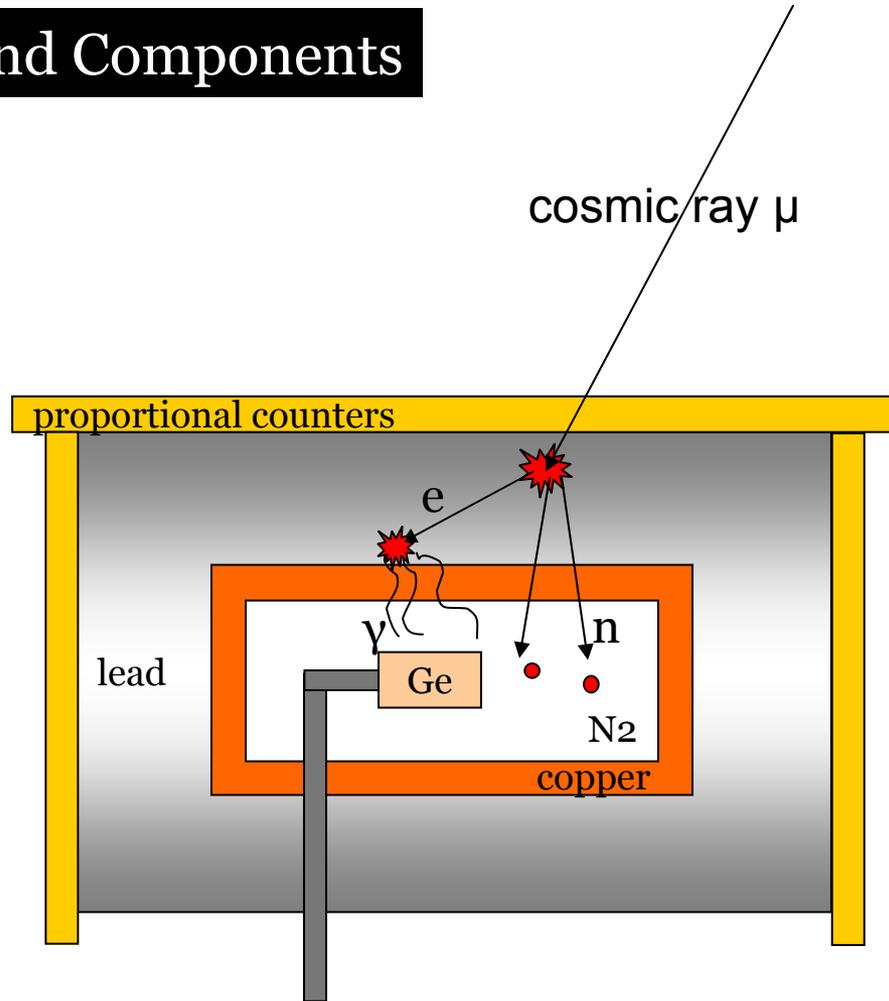
proportional chambers provide anti-coincidence veto for e.m. components
