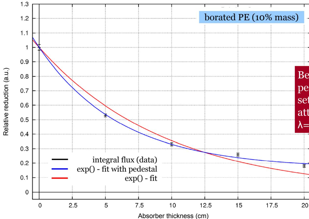
Best fit with correction for pedestal due to experimental setup yields mean attenuation length of  $\lambda = (6.2 \pm 0.6) \text{ cm}$
