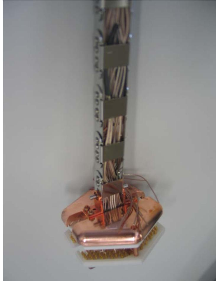
**Matrix with signal cables attached. All in cable chain**
