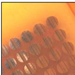
**Cables laser welded to copper pins**
