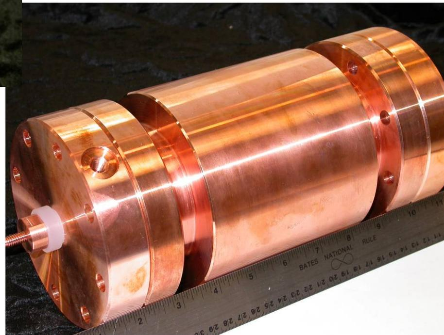
Parts are test-fit prior to cleaning and vacuum bake
