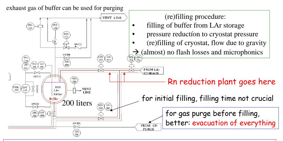
emptying: i) evaporation with heater: 2 weeks for 10 kW
