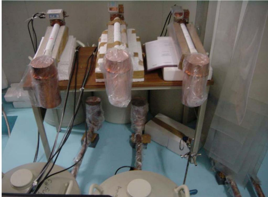
**The detectors have been put as much as possible close to each other. The three IGEX detectors were fixed on a table, with distance between them about 25 cm. The ANG 2 detector was placed at the floor below, at the distance about 50 cm from the table surface.**
