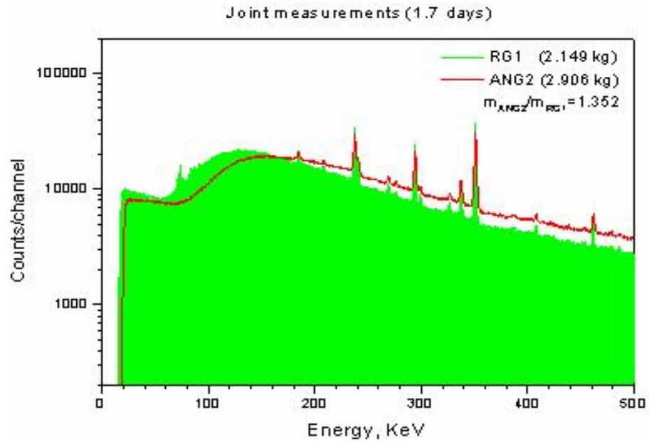
1. Low energies – shape of the spectra depend on constructions of the detectors.
