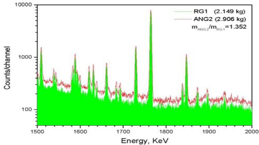
**Parts of spectra which can be used for the estimations. Peaks should be excluded. The most prominent feature of the spectra - identity of the continuum shapes.**
