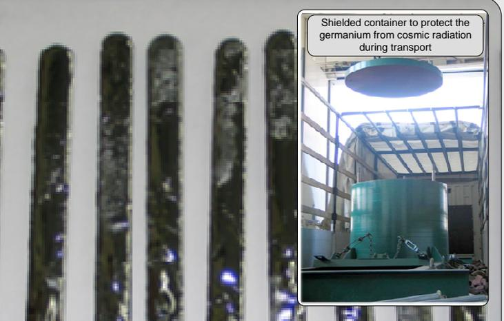
Shielded container to protect the germanium from cosmic radiation during transport
