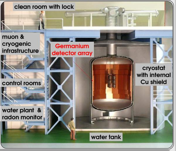
The operation of a large volume cryostat in a water tank is unique, so far. The setup accounts for all recommendations of a detailed risk analysis including earth quake tolerance up to 0.6g. The cryostat adheres to the principle of leak before break, has no penetration below the fill level and is certified for 1.5 bar overpressure being actually operated at 0.2 barg. The water tank can be completely drained within less than 2 hours.
