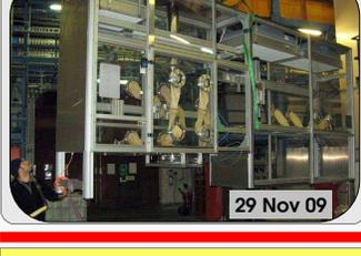
The GERDA experiment has been designed for the clean handling and the stable long-term operation of the Germanium Detector Array in a shield of liquified gas, copper and water that suppresses the environmental radioactivity by a factor of  $\sim 1/100\,000\,000$ .
