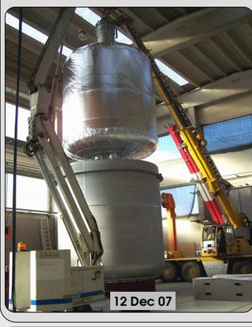
**Fotos (left)** Insertion of the cryostat's inner vessel ( $\varnothing 4.0\text{m}$ ) into the outer shell ( $\varnothing 4.2\text{m}$ ). The inner vessel is covered with „superinsulation“ to keep the thermal losses of the cryostat below 300W.
