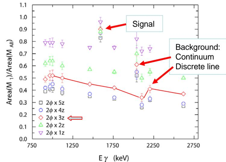
Measured with 40-fold segmented LLNL detector (data from 1 yr underground background exp.)
