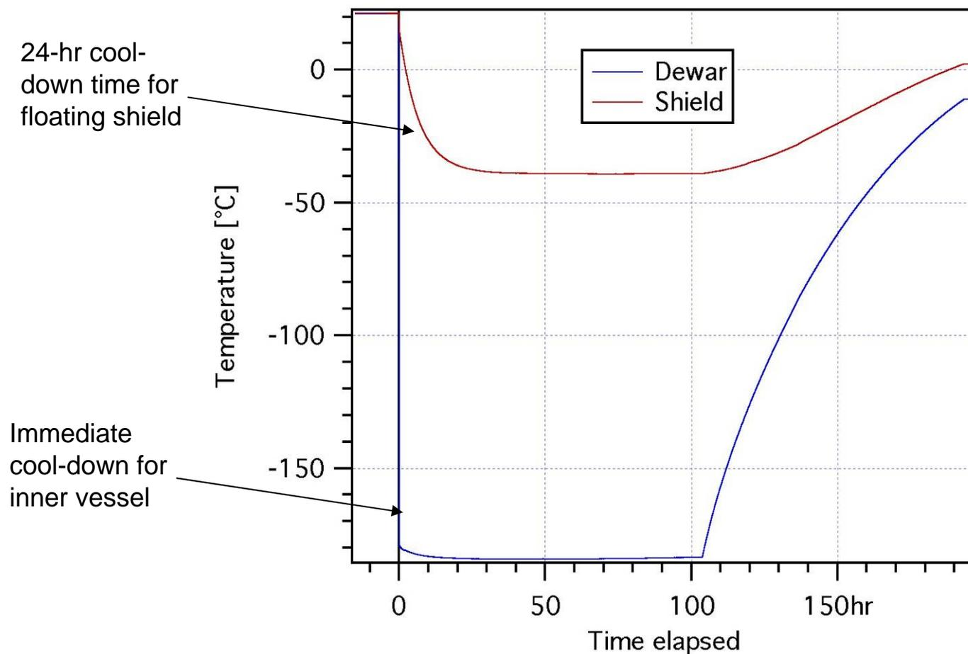
(data taken with incomplete IR shield - no coverage at bottom)
