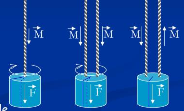
1.)Holding steel cables: Don't cause rotation !!
