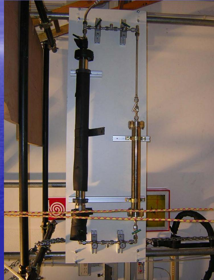
Filtration by these sieves reduces the  $O_2$  concentration
