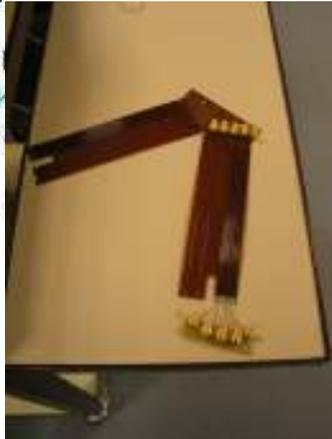
Flexible Printed Circuit Copper on Kapton
