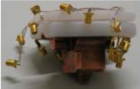
Copper Pin Plus Pogo Pin matrix on sled
