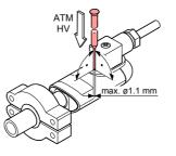
Evacuate to  $p \ll 10^4$  mbar (recommended) or to a pressure in the range of  $10^4 \dots 10^2$  mbar and wait at least 2 minutes.
