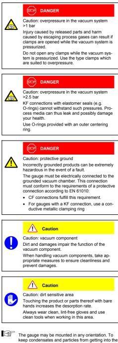
measuring chamber preferably choose a horizontal to upright position and possibly use a seal with a centering ring and filter. If adjustment should be pos-
