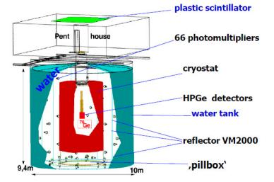
The <u>ultra-pure water buffer</u> serves as a gamma and neutron shield and as a Cherenkov detector for vetoing cosmic muons with the efficiency of more than 99 %. Plastic scintillator panels (20 m<sup>2</sup>, 20 x 2 = 40 modules)
