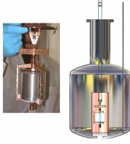
**Long-term stability tests** of naked HPGe detectors were performed in test banches filled with Liquid Argon. The detector parameters (FWHM = 2.5 - 2.9 keV at 1332 keV)do not deteriorate after one year of continuous operation in LAr even after irradiation with intensive gamma sources. This shows the feasibility of the overall GERDA project.
