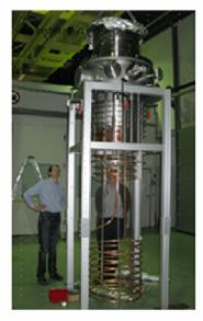
The cryostat is equipped with an active cooling system using LN<sub>2</sub> which due to sub-cooling of LAr provides minimal losses of evaporated argon  $(< 0.1 \text{ m}^3 / 10 \text{ days})$
