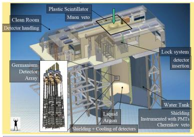
A stainless steel cryostat (25 t) with internal Cu shield (20 t) contains 90 t of liquid argon.
