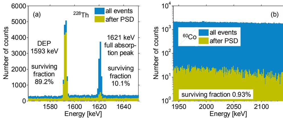
**FIGURE 3.** Recorded spectra before and after the PSD cut: (a)  $^{228}\text{Th}$  zoomed on the DEP of the 2.6 MeV line, and the 1.6 MeV FEP of  $^{212}\text{Bi}$ ; (b)  $^{60}\text{Co}$  zoomed on the energy region around  $Q_{\beta\beta}$ .
