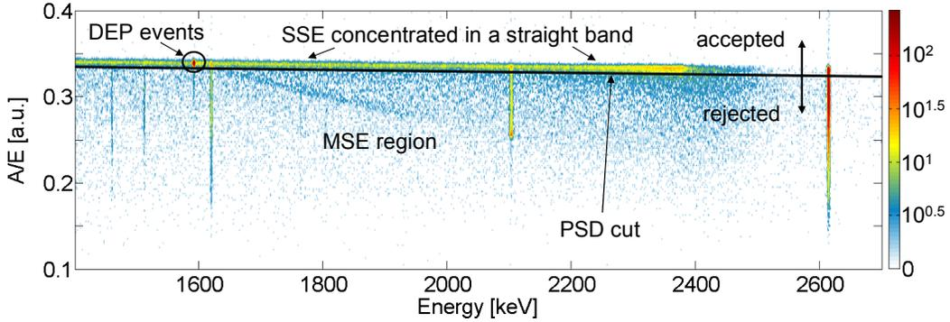
**FIGURE 2.** Density plot of the  $A/E$  parameter distribution (in arbitrary units,  $a.u.$ ) in a  $^{228}\text{Th}$  spectrum. The scale bar on the right indicates the number of events in a square of  $1\text{ keV} \times 0.0025\text{ a.u.}$
