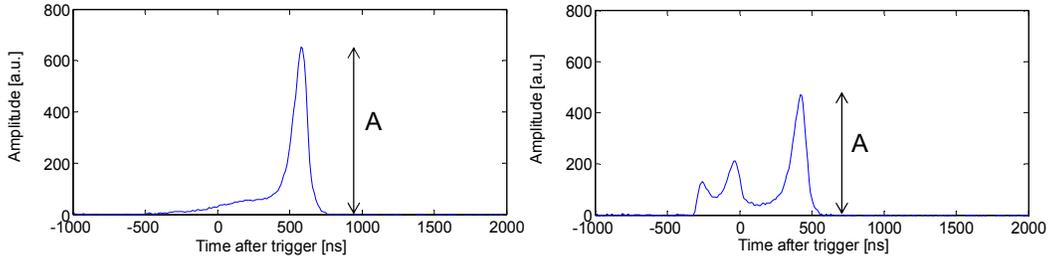
**FIGURE 1.** Candidate SSE (left) and MSE (right) current signals reproduced offline by 10 ns differentiation and 50 ns smoothing from recorded voltage signals, with an approximately equal energy. The maximal current amplitude  $A$  is proportional to the highest energy deposition within an event.
