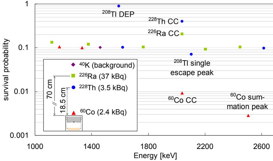
**FIGURE 4.** PSD cut survival probabilities of spectral peaks, and events from Compton continuum (CC) around  $Q_{\beta\beta} = 2039$  keV. The data points that are not full absorption peaks are labelled.
